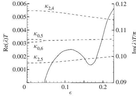
FIGURE 13. —, growth rate  $\text{Re}(\lambda)$  and ---, eigen-frequency  $\text{Im}(\lambda)$  of three-dimensional perturbations (labelled by their respective dominant components) for a non-axisymmetric base standing wave, wavenumber  $k_{1,5}$ , in a circular tank ( $h/R = 0.5$ ) plotted as a function of fundamental wave steepness  $\varepsilon$ .
