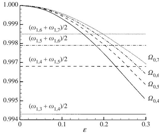
FIGURE 17. Nonlinear frequency  $\Omega_{0,\nu}$  of an axisymmetric standing wave in a circular tank ( $h/R = 0.5$ ) of wavenumber  $k_{0,\nu}$  as a function of wave steepness  $\varepsilon$ , plotted against the linear frequency combination  $(\omega_{1,\nu-1} + \omega_{1,\nu})/2$ . For each  $\nu$ , —,  $\nu = 4$ , ---, 5, — · —, 6, and  $\cdots$ , 7, the values are normalized by  $\omega_{0,\nu}$  (curves corresponding to different  $\nu$  actually do not cross).
