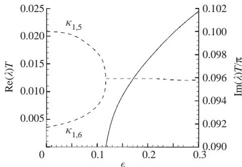
FIGURE 10. —, growth rate  $\text{Re}(\lambda)$  and ---, eigen-frequency  $\text{Im}(\lambda)$  of the perturbation containing  $(\kappa_{1,5}, \kappa_{1,6})$  for the axisymmetric standing wave  $k_{0,6}$  in a circular tank ( $h/R = 0.5$ ) as a function of the fundamental wave steepness  $\varepsilon$ .
