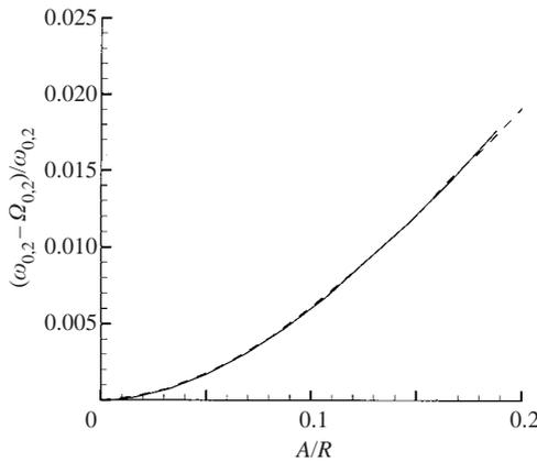
FIGURE 3. Frequency  $\Omega_{0,2}$  of nonlinear axisymmetric standing wave  $k_{0,2}$  in a circular tank (with  $h/R = 1.0$ ), normalized by  $\omega_{0,2} = (gk_{0,2} \tanh k_{0,2}h)^{1/2}$ , as a function of the wave amplitude  $A/R$ . ---, fully nonlinear result of Tsai & Yue (1987); —, present HOSE simulation (with  $M = 3$ ).
