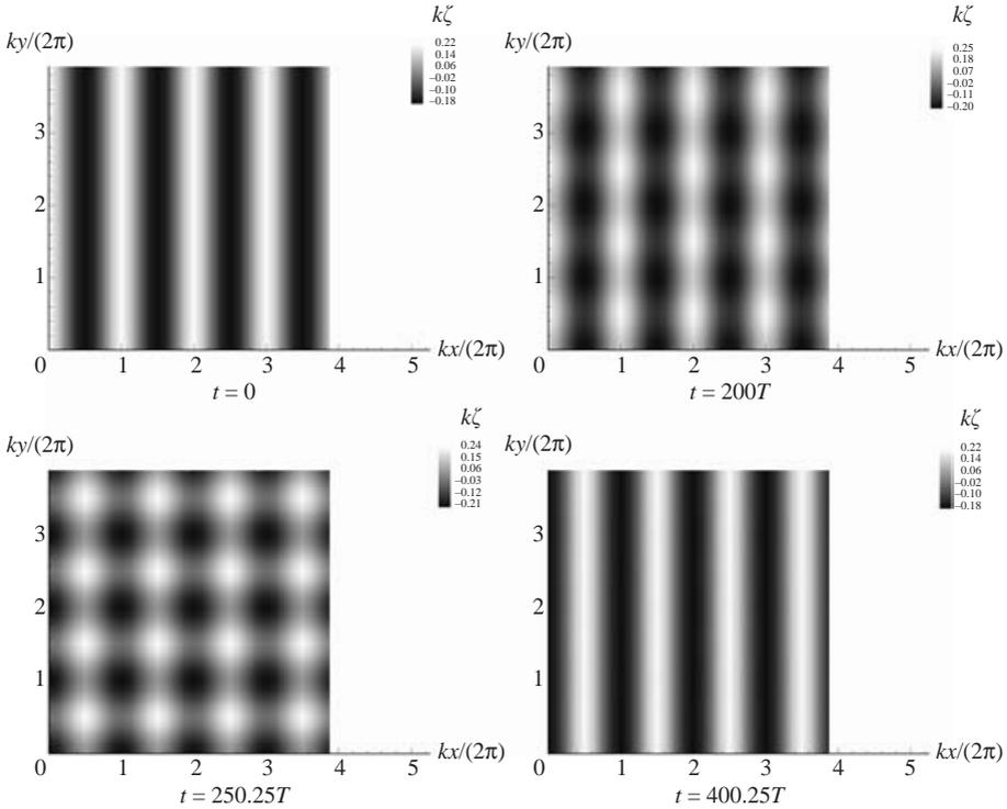
FIGURE 9. Snapshots of the free surface during the nonlinear evolution of a plane standing wave  $kA = 0.20$  initially perturbed by an unstable transverse wave (with  $\mathcal{L} = 4$ ,  $\mathcal{W} = 4.04$ ,  $p = 0$ ,  $q = 4$ ).
