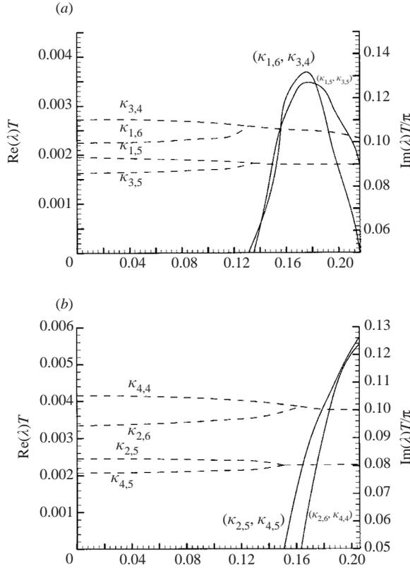
FIGURE 14. —, growth rate  $\text{Re}(\lambda)$  and ---, eigen-frequency  $\text{Im}(\lambda)$  of three-dimensional perturbations (labelled by their dominant components) for non-axisymmetric base standing waves with (a) wavenumber  $k_{2,5}$  and (b)  $k_{3,5}$  in a circular tank as a function of the fundamental wave steepness  $\epsilon$ .
