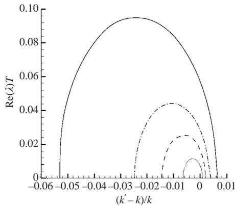
FIGURE 6. Growth rate of a transverse ( $\alpha = 90^\circ$ ) unstable mode on a plane standing waves of  $\cdots$ , wave steepness  $kA = 0.10$ ;  $---$ ,  $0.15$ ;  $-\cdot-$ ,  $0.20$ ; and  $—$ ,  $0.30$ .
