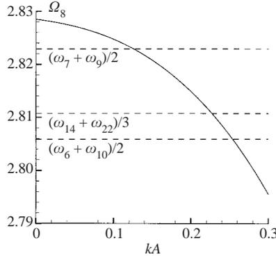
FIGURE 16. Nonlinear frequency  $\Omega_8$  of the plane standing wave  $k_8$  as a function of the wave steepness  $kA$ , plotted with the linear frequency combinations  $(\omega_7 + \omega_9)/2$ ,  $(\omega_6 + \omega_{10})/2$  and  $(\omega_{14} + \omega_{22})/3$ . The plotted frequencies are normalized by  $\omega_1$ .
