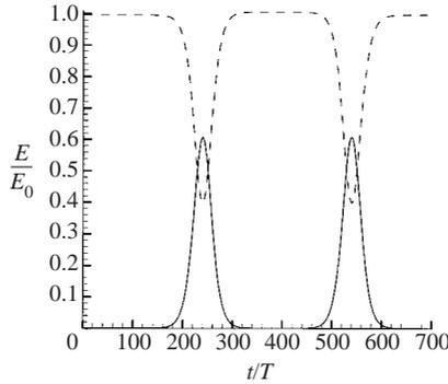
FIGURE 8. Time history of total wave energy  $E$  (normalized by the initial energy of the fundamental wave  $E_0$ ) during nonlinear evolution of a plane standing wave  $kA = 0.20$  initially disturbed by an unstable transverse perturbation (with  $\mathcal{L} = 4$ ,  $\mathcal{W} = 4.04$ ,  $p = 0$ ,  $q = 4$ ) for: ---, the fundamental standing wave; —, the transverse mode.
