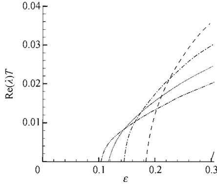
FIGURE 11. Growth rates of the perturbation containing  $(\kappa_{1,\nu}, \kappa_{1,\nu-1})$  for axisymmetric standing waves  $k_{0,\nu}$  in a circular tank ( $h/R = 0.5$ ) as a function of the fundamental wave steepness  $\varepsilon$ . The plotted curves are for: —,  $\nu = 3$ ; ---,  $\nu = 4$ ; - · - ·,  $\nu = 5$ ; · · ·,  $\nu = 6$ ; — · — ·,  $\nu = 7$ .
