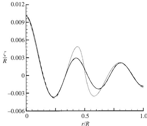
FIGURE 1. Free-surface profiles of nonlinear axisymmetric standing wave  $k_{0,6}$  in a circular tank at  $t = 0$  (corresponding to maximum elevation of this standing wave profile at the origin) obtained with:  $\cdots$ ,  $(N_{FE}, N_{Fr}) = (2, 4)$ ;  $---$ ,  $(4, 4)$ ;  $- \cdot -$ ,  $(4, 8)$ ;  $—$ ,  $(4, 16)$ . The wave amplitude  $A/R = 0.01$ . ( $M = 3$ ,  $N_{F\theta} = N_{w\theta} = N_{b\theta} = 16$ ,  $N_{wz} = N_{br} = 16$ ,  $T/\Delta t = 128$ ,  $h/R = 0.5$ .)
