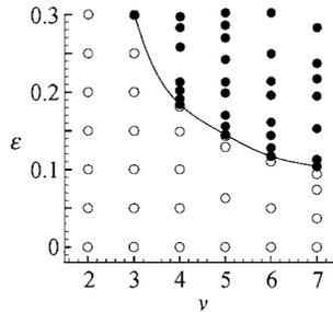
FIGURE 12. Region of (in)stability for axisymmetric standing waves  $k_{0,\nu}$  as a function of  $\nu$  and fundamental wave steepness  $\varepsilon$ . ○, stable; ●, unstable standing waves.
